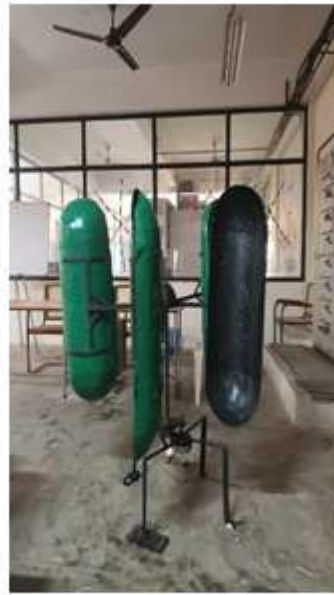
Fig.8. Finished vertical axis wind turbine
